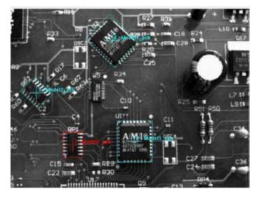
Sapera Search Tool supports rotation independent, simultaneous multiple target detection.
